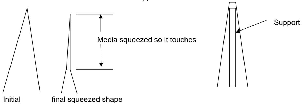
The support can be a laminate that is stiff but a very open media. This allows the use of virtually any media in pleated construction.
