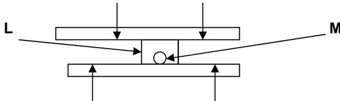
A resilient seal, labeled L is placed between the sealing service presumably round, and at 120 degree intervals the seal is slit and a ball bearing, labeled M, is dropped into the slot. This maintains sufficient sealing pressure but does not allow over compression of the seal. Other stops can be incorporated into the mounting system.
